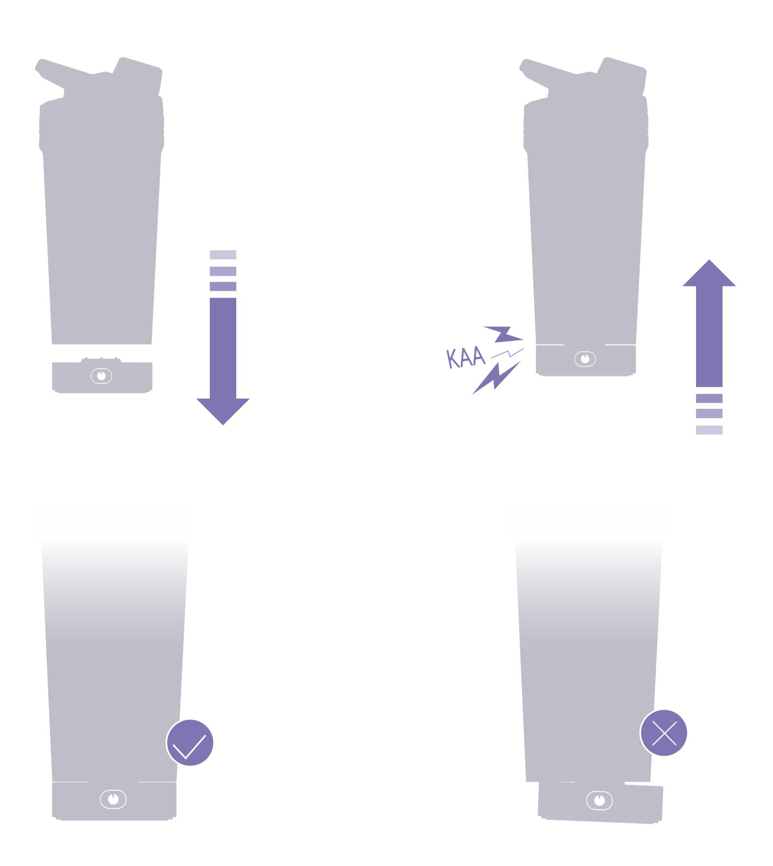
Proper installation: The body and the base are tightly fitted together.
